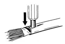
5.04 Place bond conductor (strap, bar, wire, or braid) over stud and secure in place with nut supplied. Torque nut to 40-50 in-lbs (5.2±0.6 kgm) with company approved tool.
