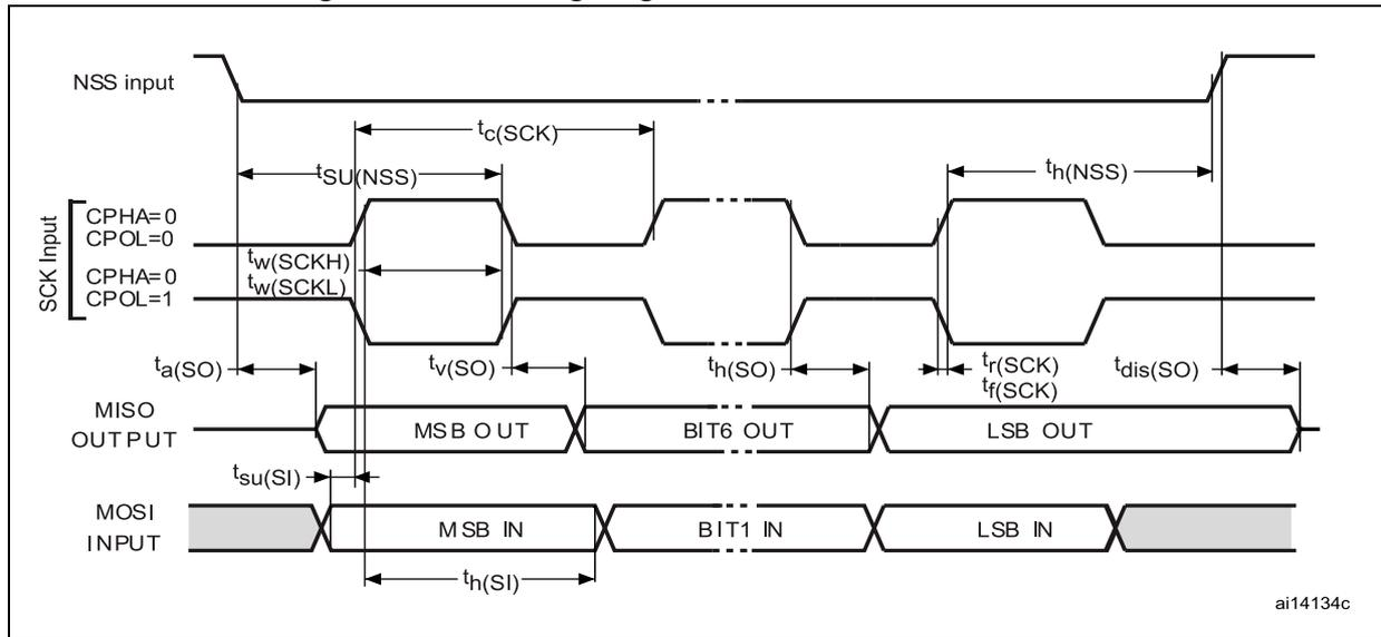
Figure 26. SPI timing diagram - slave mode and CPHA = 1<sup>(1)</sup>
