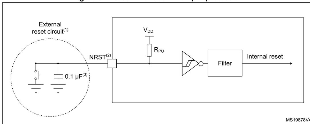
1. The reset network protects the device against parasitic resets. 0.1 uF capacitor must be placed as close as possible to the chip.
