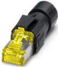
RJ45 connector, IP20, CAT6<sub>A</sub>, 8-pos., with QUICKON fast connection technology, for 26 ... 24 AWG 1-wire and 7-wire conductors, color: black
