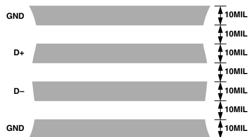
Figure 5. Arrangement of Signal Tracks
