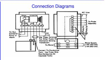
Model LCT is a forward mode control. The control relay is energized when liquid rises to contact the "H" probe. The time delay on operate is 3 seconds nominal and 0.5 seconds on release. Other values between 0.5 and 10 seconds are available on request. The control relay is pulled in and remains energized until liquid drops below the "L" probe. Sensitivity is adjustable.
