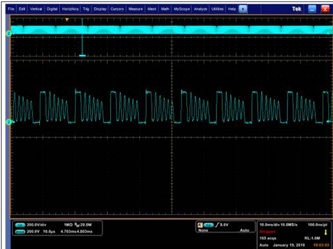
Figure 18. 230 VAC Valley Switching 100-mA Load
