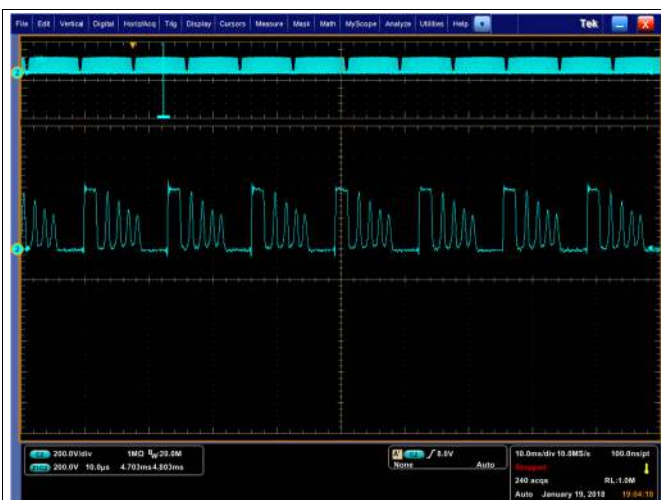
Figure 16. 85 VAC Valley Switching 50-mA Load
