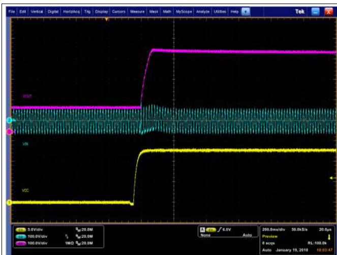
Figure 7. 85 VAC Start-up No Load
