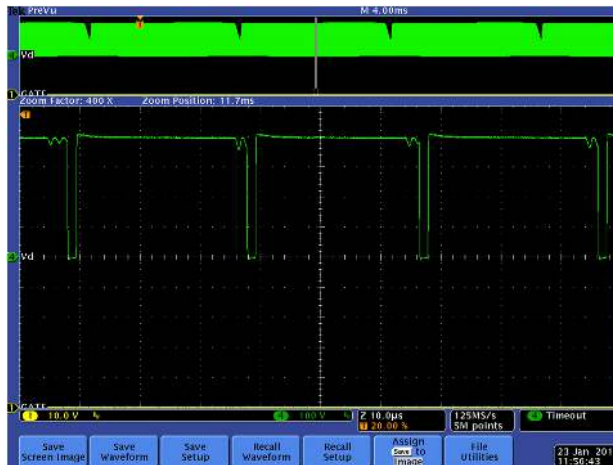
Figure 21. D4 Max Voltage Stress
