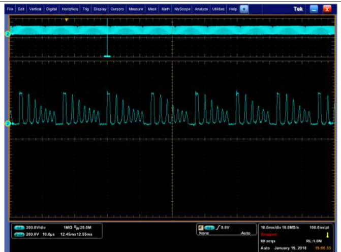
Figure 19. 265 VAC Valley Switching 100-mA Load
