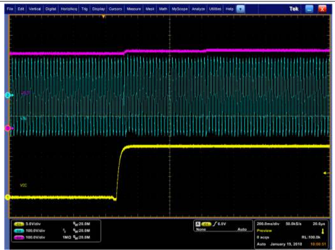
Figure 12. 265 VAC Start-up No Load
