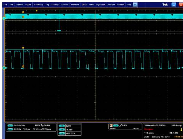
Figure 20. Q1 Max Vds Stress
