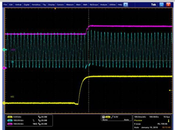
Figure 10. 230 VAC Start-up No Load
