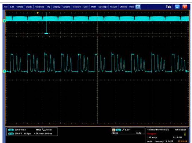
Figure 17. 115 VAC Valley Switching 50-mA Load
