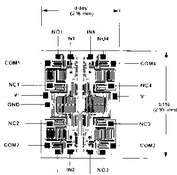
NOTE: NCx IS CONNECTED TO COMx WHEN INx IS LOW.
