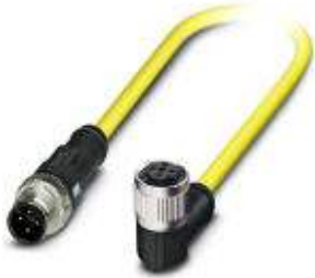
Sensor/Actuator cable, 4-position, TPE, yellow RAL 1021, Plug straight M12 SPEEDCON, A-coded, on Socket angled M12 SPEEDCON, A-coded, Cable length: 3 m
