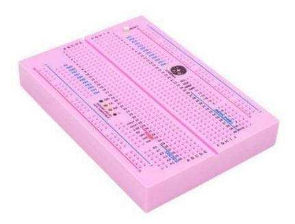
**Description:** The STEMTera is an innovation in breadboard history. It is the first breadboard with an Arduino-compatible hardware suite built in that works with thousands of shields. With ATmega16U2/32U2 pins exposed, native USB projects can be easily developed using the LUFA framework. The STEMTera also features a LEGO® brick-compatible bottom that empowers projects to be built beyond imagination. This version of the STEMTera is housed in a durable pink ABS plastic enclosure.
