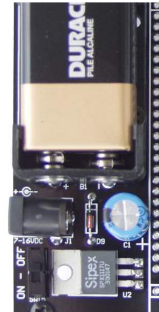
Figure 9: The Decoder Board Power Supply Area
