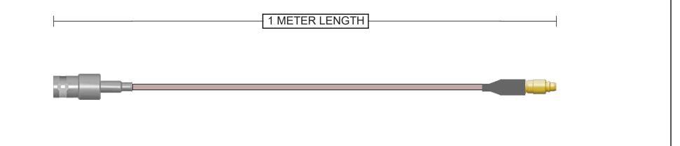
Connector A 112160 BNC Jack Straight Brass Nickel 50 Ohm RG-316 Continuity/Hi-Pot Connector B 262101 MMCX Plug Straight Brass Gold + Heatshrink
