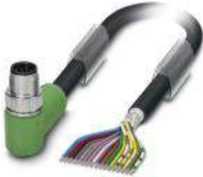
Sensor/Actuator cable, 17-position, PUR/PVC, Black RAL 9005, shielded, Plug angled M12-SPEEDCON, A-coded, on Free cable end, Cable length: 5 m
