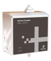
The 2510 and 2510-2 particle counters provide a range of particle size measurement from 0.5 to 5.0  $\mu$ m at a flow rate of 1.0 CFM (28.3 LPM). These sensors allow for efficient particle counting with specifications that exceed the ISO 21501-4 and JIS B9921 calibration standards.
