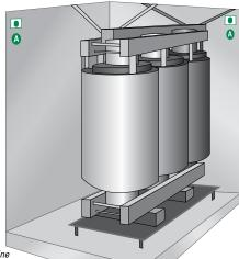
Place sensors in direct line of sight to possible arc faults, preferably pointing down from the ceiling.
