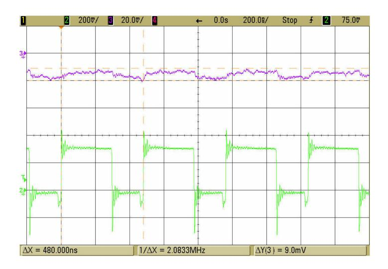
Figure 3. Switch Node & Output Ripple Voltage Waveforms  $V_{IN} = 3.3V, \ V_{OUT} = 1.8V, \ I_{OUT} = 4A$
