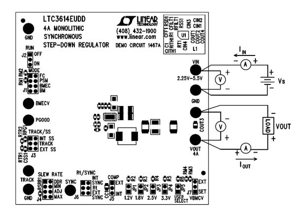
Figure 1. Proper Measurement Equipment Set-Up
