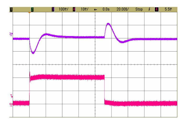
Figure 4. Load Step Response  $V_{IN}$  = 3.3V,  $V_{OUT}$  = 1.8V, 4A Load Step (0.1A <-> 4A)
