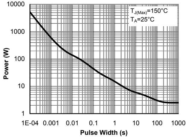
Figure 15: Single Pulse Power Rating Junction-to-Ambient (Note G)
