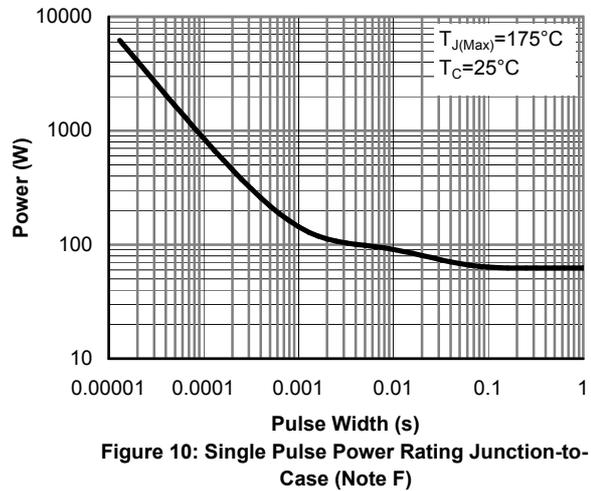
Figure 10: Single Pulse Power Rating Junction-to-Case (Note F)
