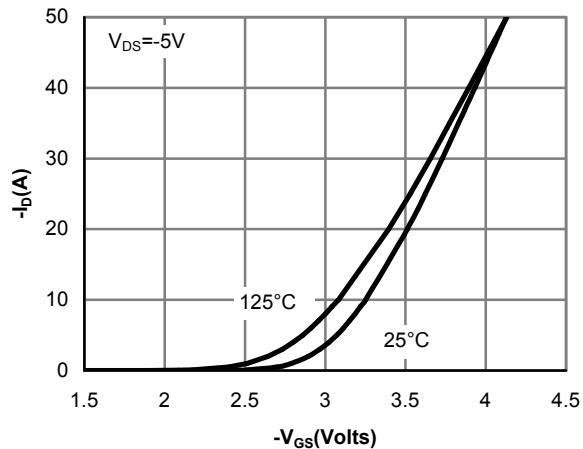
Figure 2: Transfer Characteristics
