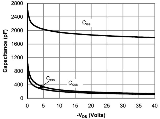
Figure 8: Capacitance Characteristics
