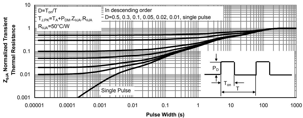
Figure 16: Normalized Maximum Transient Thermal Impedance (Note G)
