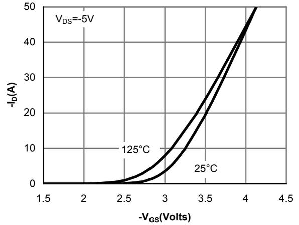
Figure 2: Transfer Characteristics
