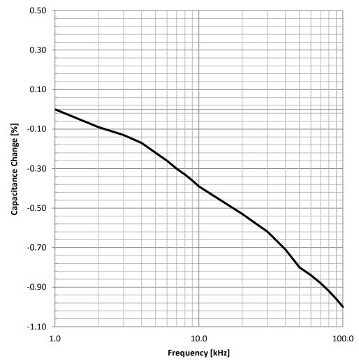
Test Equipment: E4991A or equivalent
