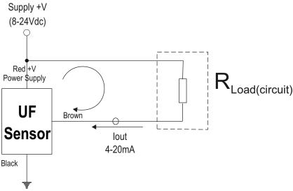
An ammeter (or suitably arranged multi-meter), placed in series at the lout point, will give an indication of the sensors current performance i.e.
