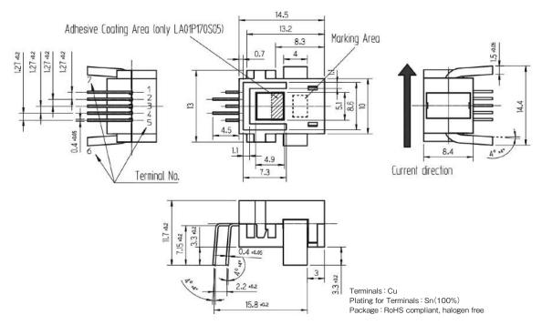
Note1) The tolerances of dimensions without any mention are ± 0.1mm. Note2) The adhesive material (RoHS compliant, halogen free) is used for holding the magnetic core. (Only LA01P170S05)
