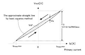
$\cdot$  When Ip\_{(RMS)}max is bigger than the value of If, Ip\_{(RMS)}max restricts it to the value of If.
