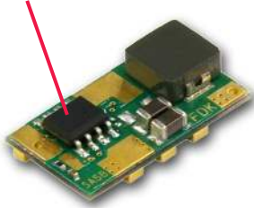
Fig. E: Location of the thermocouple for thermal testing
