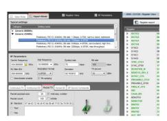
You can now configure the radio, performance tests, export register settings and run link tests with another CC1200 or CC1201 on a SmartRF TrxEB connected to the PC.
