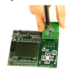
Insert a CC120xEM board into the TrxEB as shown above. Connect the antenna to the SMA connector on the EM.
