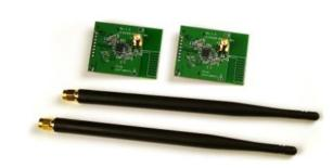
2 x CC1200 or CC1201 Evaluation Modules 2 x Antennas (type depending on frequency)
