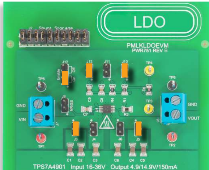
Figure 6. TPS7A4901 LDO board: jumpers set-up for Test#1
