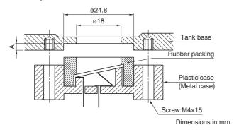
The transducer can beak off if the A dimension depth is shallow. TDK recommends a 2mm A-dimension depth and a screw tightening torque of 0.39N • m.
