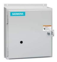
Non-reversing contactor, Size 2 1/2, Three phase full voltage, Contactor amp rating 60A, 3 wire (NO aux included), 220-240/440-480VAC 60Hz coil, Non-combination type, Enclosure NEMA type 12, Dust/drip proof for indoors, Extra-wide enclosure
