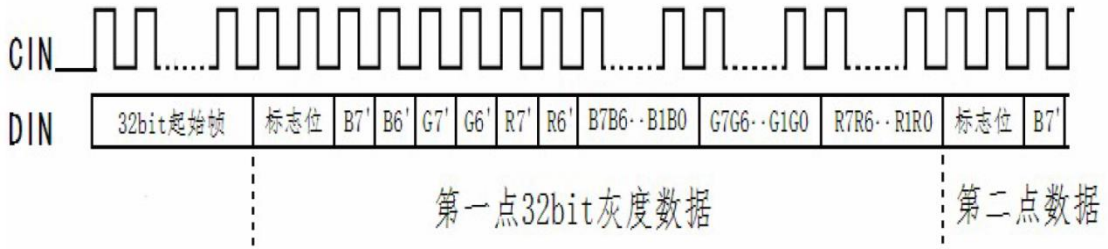
Figure 3.3 P8913 Driving sequence diagram
