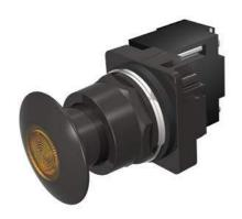
30mm BlackMax, Epoxy Coated Corrosion Resistant Complete Metal Unit Illuminated Push-Pull Operator Full Voltage, 12V AC/DC Incandescent Lamp Mushroom Head Cap Small 1 3/4" (44.5 mm) Metal, Black with Amber Lens 3 Position Momentary UL Listed, CSA Certified NEMA 1,3,3R,4,4X,12,13 & Automotive Standards
