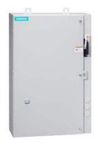
Non-reversing motor starter, Size 3, Three phase full voltage, Solid-state overload relay, OLRelay amp range 25-100A, 24VAC 50-60HZ coil, Combination type, 100A non-fusible disconnect, Enclosure NEMA type 4/12, Water/dust tight for outdoors, Standard width enclosure
