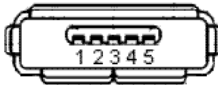
Figure 6-6. USB Host/Device Micro AB connector J14
