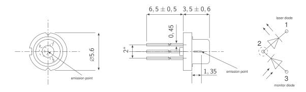
all dimensions in mm. Tolerance  $\pm 0,\,2$  except given ones \* at the bottom of the LED
