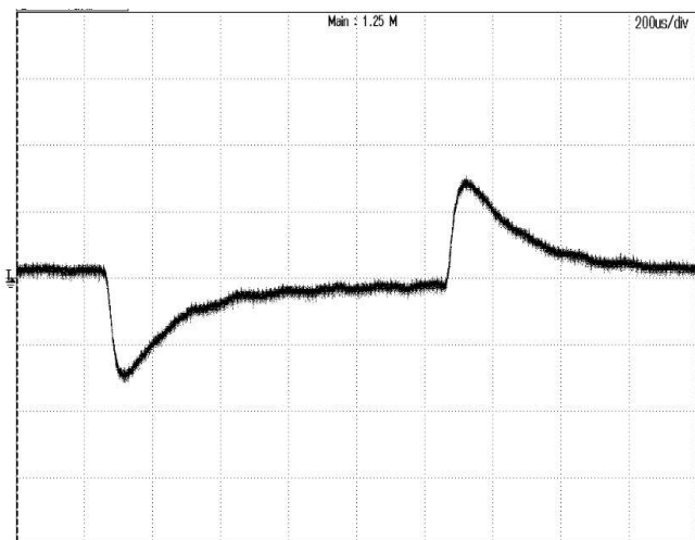
Figure 5: Output voltage response to step-change in load current (50%-75%-50% of full load; di/dt = 0.1A/\mu s ). Trace: Vout: 200mV/div; Time: 200us/div
