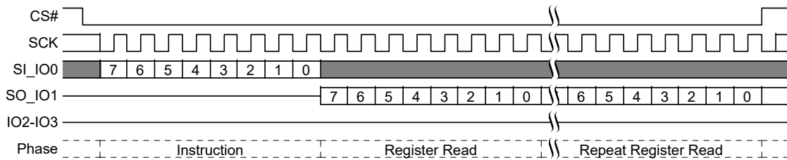
Figure 56. Read Configuration Register (RDCR) Command Sequence
