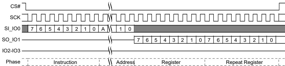
Figure 110. PPB Read Command Sequence
