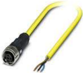
Sensor/Actuator cable, 3-position, TPE, yellow RAL 1021, free cable end, on Socket straight M12 SPEEDCON, A-coded, Cable length: 10 m
