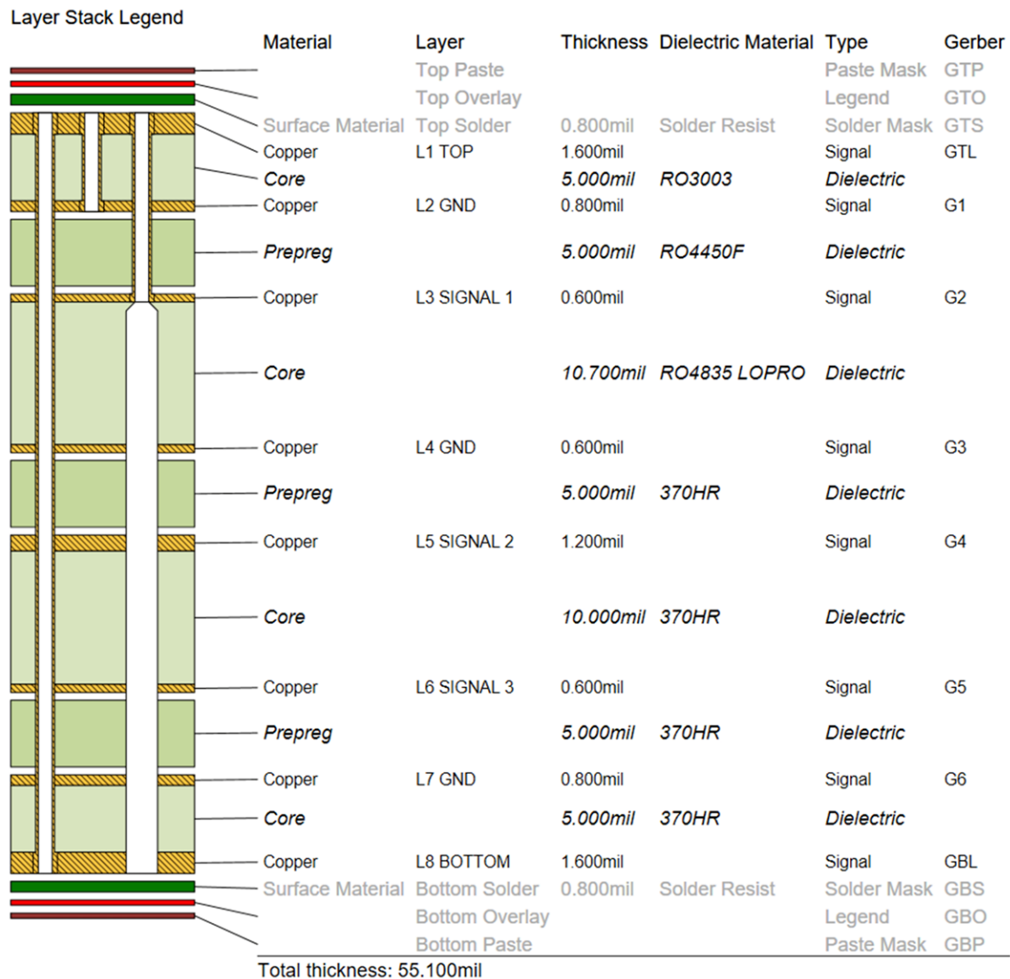
Figure 30. MMWCAS-RF-EVM PCB and Drill Stack-Up Table
