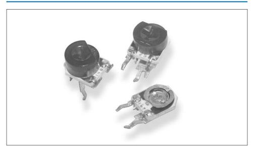
This tiny 6mm square cermet trimmer is offered with alternative adjustment covers for screwdriver and automatic setting and can be supplied in bulk or taped in ammo pack. The 416 can be adjusted from the top or side and is an inexpensive solution to high reliability potentiometer requirements. This series is used to replace some of the larger, expensive, sealed types in high volume circuits.
