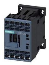
traction contactor, AC-3e/AC-3, 12 A, 5.5 kW / 400 V, 3-pole, 24-34 V DC, 0.7-1.25\* Us, electronic drive, with integrated varistor, auxiliary contacts: 1 NC, spring-loaded terminal, size: S00
