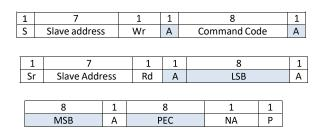
**Block communications:** When writing or reading more than two bytes of data at a time BLOCK instruction for WRITE and READ commands are used instead of the Standard Instructions above to write or read any number of bytes greater than two.
