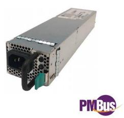
The MPR0712 series is a 700W ACDC power supply with a power density of 23W/in3 at an efficiency of 94% @ 50% Load. The smaller depth of 9" would be conducive for mid plane system architectures and in applications that are limited in space. MPR0712 uses the industry standard PMBus<sup>®</sup> compliant I2C communications bus and offers a full range of control and monitoring capabilities. The SMBAlert signal pin automatically alerts customers of any state
