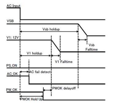
Power removal holdup, fall time and signaling
