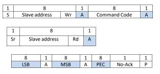
Read back error: If the  $\mu$ C does not have sufficient time to retrieve the requested data, it has the option to return all FF's instead of incorrect data.
