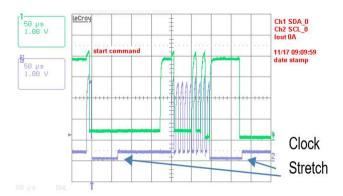
**I<sup>2</sup>C Bus Lock-Up detection:** The device will abort any transaction and drop off the bus if it detects the bus being held low for more than 35ms.
