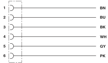
Contact assignment of the DEUTSCH DT06-6S
