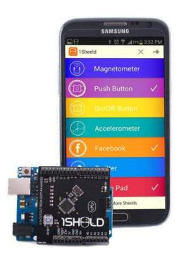
1Sheeld turns your smartphone into a re-configurable Arduino shield
