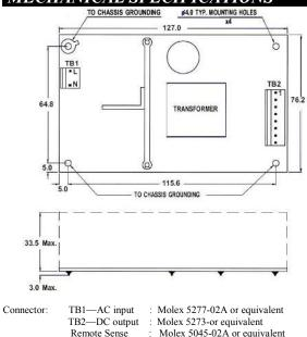
Size: 76.2mm X 127mm X 33.5mm, 3" X 5" X 1.319" Mounting Holes: 64.8mm X 115.6mm, 2.55" X 4.55"
