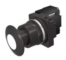
30mm BlackMax, Epoxy Coated Corrosion Resistant Complete Metal Unit Illuminated Push-Pull Operator Full Voltage, 12V AC/DC Incandescent Lamp Mushroom Head Cap Small 1 3/4" (44.5 mm) Metal, Black with White Lens 3 Position Pull-Momentary/Push-Maintained UL Listed, CSA Certified NEMA 1,3,3R,4,4X,12,13 & Automotive Standards
