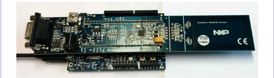
Fig 14. CLEV663B connected to LPCXpresso LPC11U68 development board
