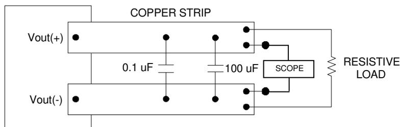
Note: Use a 0.1 $\mu$ F X7R ceramic capacitor and a 100 $\mu$ F @ 6V3 ceramic capacitor. Scope measurement should be made using a BNC socket. Position the load 3 in. [76mm] from module.
