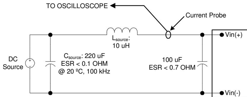
Note: Measure input reflected-ripple current with a simulated source inductance ( $L_{test}$ ) of 10  $\mu$ H. Capacitor  $C_s$  offsets possible source impedance.
