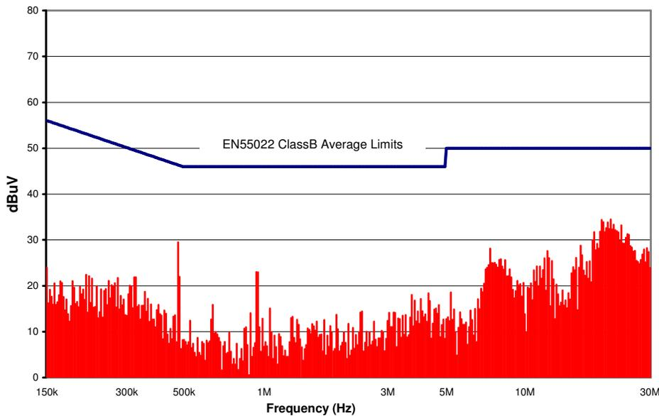
Figure 19. CPT15F18 Conducted Emissions using above specified input filter.
