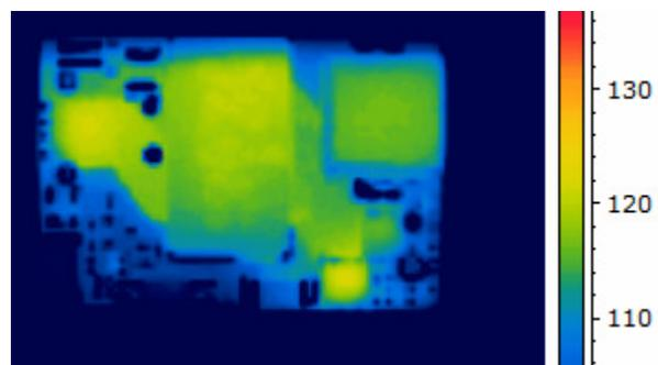
Figure 6. Thermal Image of CPT15F18 (15A output, 70C Ambient, 200lfm airflow, Vin = 18V, airflow from pin 3 to pin 1, Tmax = 122°C)
