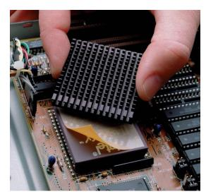
Bergquist CPU Pad is a thermally conductive, electrically insulating, double coated tape. The tape consists of a high performance acrylic, pressure sensitive adhesive, on both sides of a film. This product can be used in applications that currently require clips. CPU Pad is typically used to mount a heat sink on top of a central processing unit on the circuit board.
