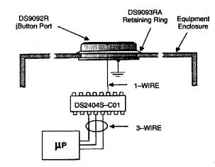
Equipment fitted with 1-Wire button contact.
