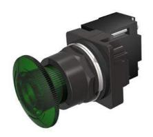
30mm BlackMax, Epoxy Coated Corrosion Resistant Metal Operator, Round Illuminated Twist-to-Release Transformer type, 600V AC LED Lamp Mushroom Head Cap Small 1.79" (45 mm) Plastic Cap, Green 2 Position Maintained, Twist-to-Release UL Listed, CSA Certified NEMA 1,3,3R,4,4X,12,13 & Automotive Standards
