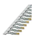
Crimp contact, Socket, rolled, Taped articles, number of pieces per reel: 500, contact diameter: 1 mm, crimp range:  $0.08~\text{mm}^2$  ...  $0.22~\text{mm}^2$
