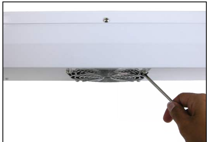
Figure 10. Shorting the ionizer’s two fan grills
