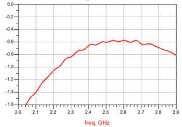
Figure 3. Insertion loss (dB)
