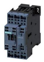
power contactor, AC-3e/AC-3, 25 A, 11 kW / 400 V, 3-pole, 24 V DC, with plugged-in varistor, auxiliary contacts: 1 NO + 1 NC, spring-loaded terminal, size: S0  $\,$
