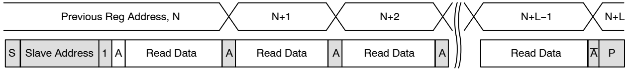
Figure 21. Sequential READ, Start from Current Location
